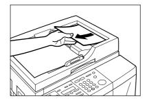
**2** Open the feeder cover and gently remove the jammed paper from the ADF.
